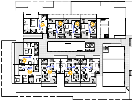
01 Ground Floor SolarVent 1:500
